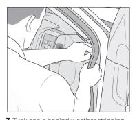
**7.** Tuck cable behind weather stripping, and push stripping in to secure it.
