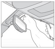
**6.** Remove adhesive and apply cable clips to windshield. Slide the bracket power cable into clips.
