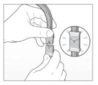
**8.** At the end of the bracket cable (A), connect the terminal to the smaller end of the adapter cable (F).
