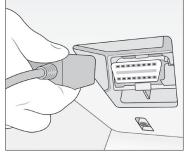
**9.** Plug the end of the OBDII adapter cable into your vehicle's OBDII port.
