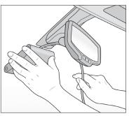
**5.** Remove backing. Press evenly to ensure the mounting bracket's adhesive is flush against the glass. Hold to window for 30 seconds.
